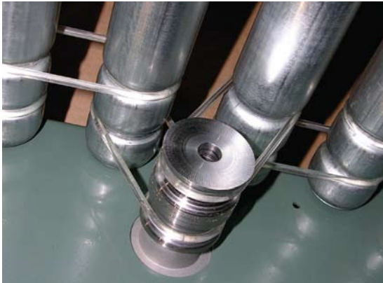
Rollers are powered by 24 VDC motors. The rollers are driven from the motor with o-rings.
