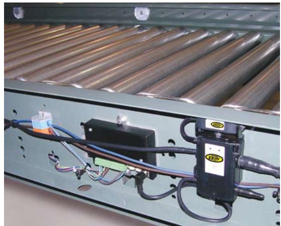
Each zone is powered by a 24 VDC motor. The rollers in that zone are driven from the motor with o-rings.
