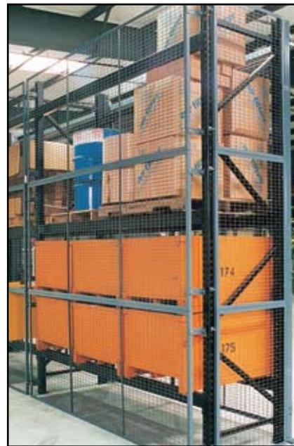
Racks can be secured with wire mesh panels that can be outfitted with lockable doors for access at the ground level. Besides security, this method can enhance safety by preventing product spillage.
