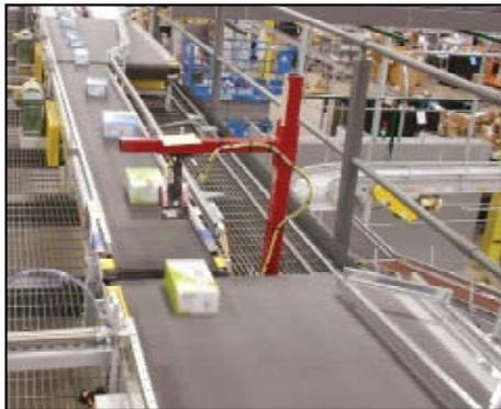
a gap so cases can enter the system individually. The system confirms information such as weight, dimension, data from a barcode and/or RFID tags, or data from vision systems. Based on the data, the case is accepted or rejected, and a number of exception process steps can occur based on your needs.
