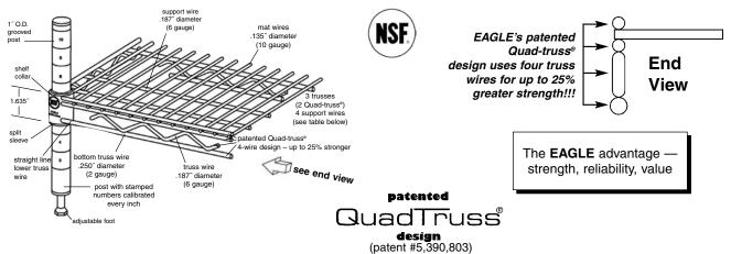
The patented Quad-truss® system makes EAGLE wire shelving products the strongest in the industry.
