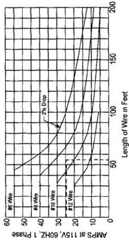
Example 1.5HP, 115V, 1 phase, 24A motor, length of wire run is 55FT. Wire size above point of intersection is #12.
