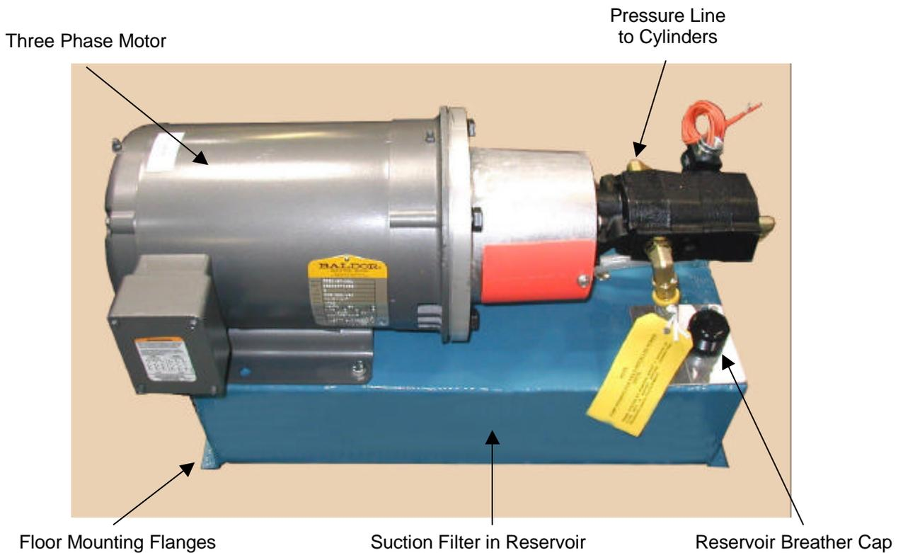
NOTE: Model 6100 Power Unit is pre-wired to a controller mounted above the motor (not shown)
