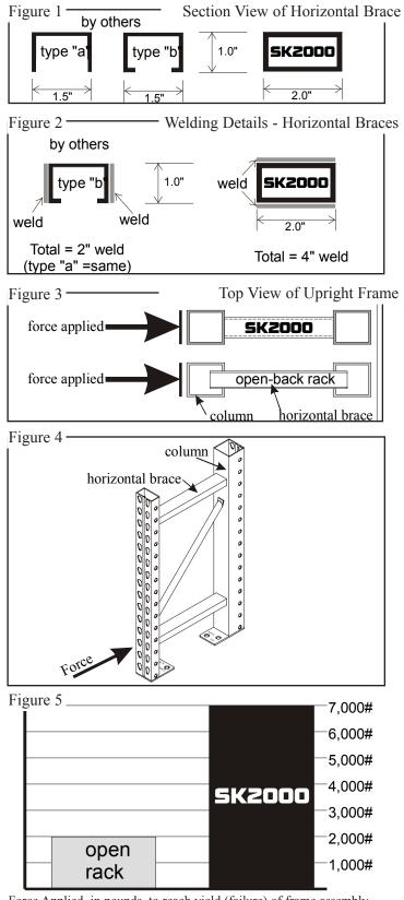
Force Applied, in pounds, to reach yield (failure) of frame assembly.
