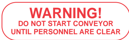
PLACED ON ALL POWERED CONVEYORS NEAR DRIVE AND/OR CONTROLS.
