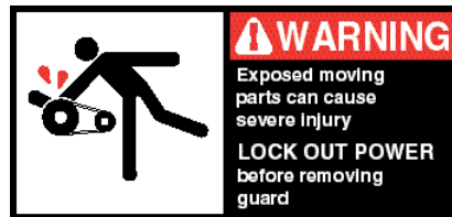
PLACED ON ALL CHAIN GUARDS.
