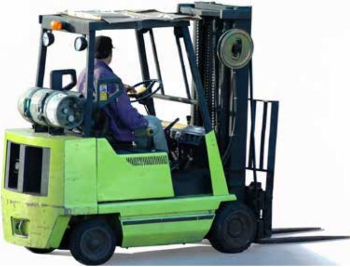
A 5,000-pound forklift moving through a warehouse at ten miles per hour with a 4,000-pound load has a potential destructive force of 135,000-foot pounds of energy. That's equivalent to a large car driving at 20 miles per hour. Even at very low speeds, forklift collisions are devastating—or fatal—to pedestrians. Forklifts take an incredible toll on equipment and buildings when they collide with storage racks, building columns, machinery — or each other.
