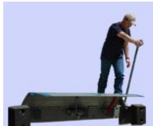
**Step 4:** Continue to push forward until the front lip rests fully on the truck bed.
