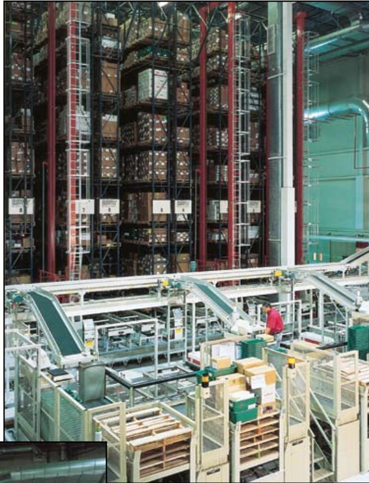
of materials, RTS directs the AS/RS to retrieve needed pallets and transport them via an STV to one of three replenishment pick stations. A picker takes the replenishment stock from the pallet, places it into a tote and attaches a bar code label. Hytrol conveyors send the tote to the correct order-picking area for restocking, and the picked-from pallet is re-stored by the AS/RS.
