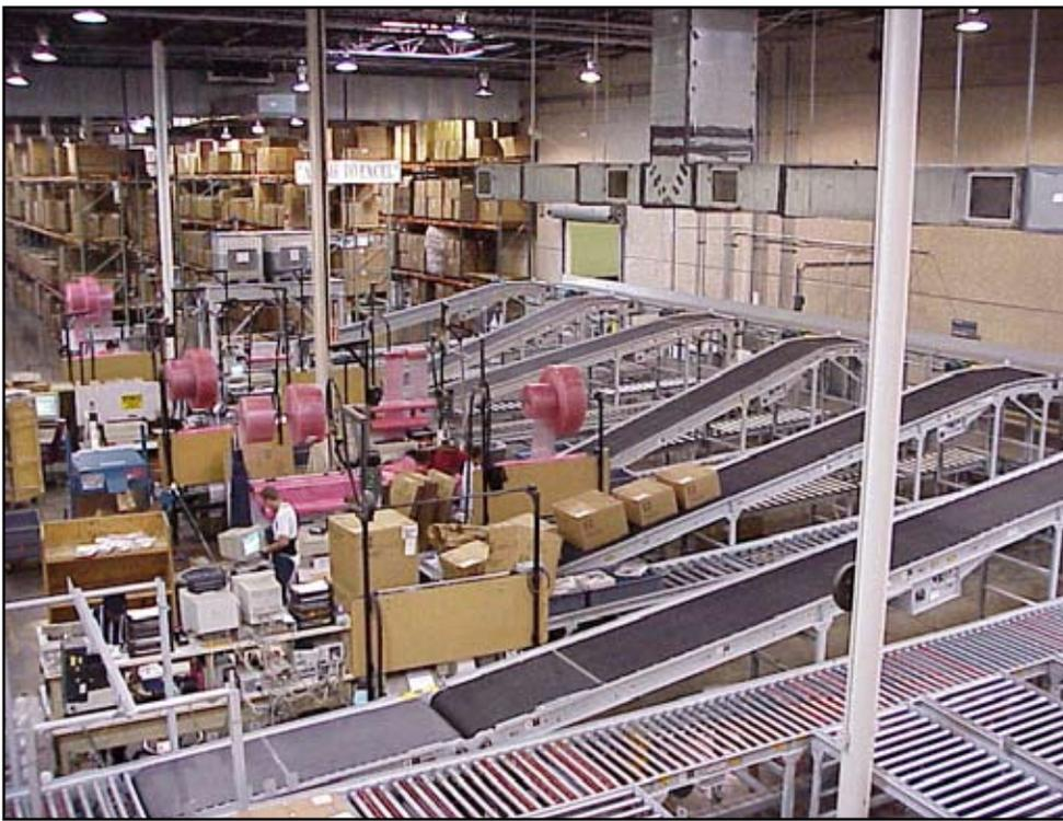
trol EZ-Logic conveyor accumulates the totes before the ship-sort system.
