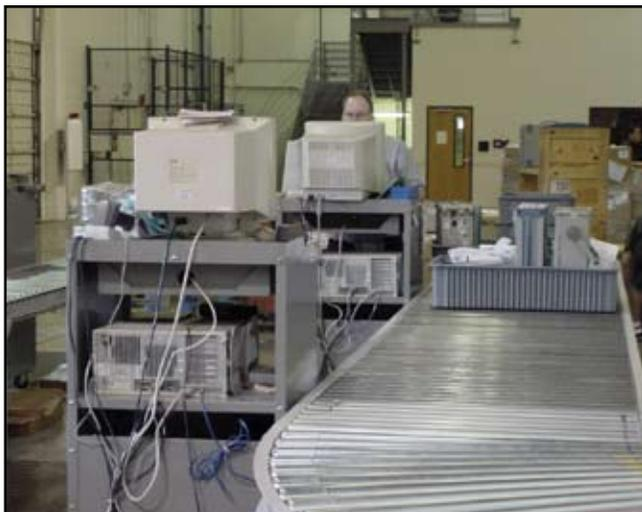
There are five incline takeaway conveyors. One is shared between each pair of pack stations. Packers can individually generate a shipping label at their stations, eliminating the need for a downstream manifest station.
