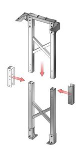
STEP 1: Orient components as needed for the desired tower height.
