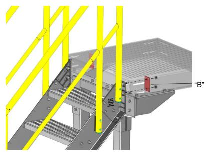
With the stair assembly fully assembled (in this configuration, tower supported) no stair to platform bracket is required), properly locate the stair unit on the pad layout anchor bolts "A".
