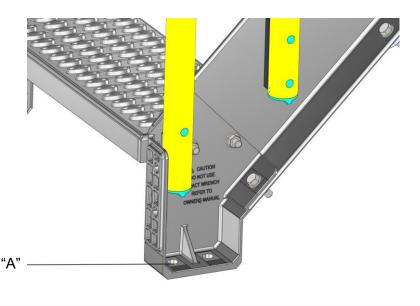
With the stair assembly fully assembled, properly locate the stair unit on the pad layout anchor bolts "A".
