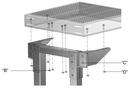
When a platform is being supported by a tower support at the stair location, the tower should be first located on the anchor bolts and secured in the final assembly location.
