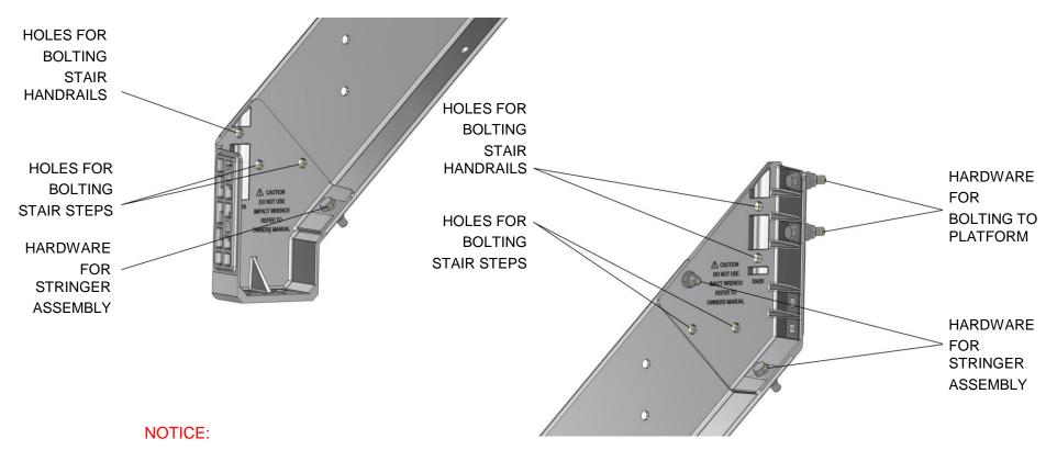
Some holes are used to connect both casting to stringer as well as connect stair steps and/or handrails.
