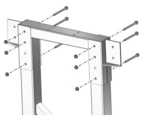
STEP 4: Attach hardware and tighten as shown.
