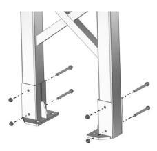
STEP 2: Attach hardware as shown and tighten hardware.
