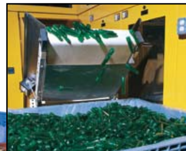
Above: Conveyor feeding bulk parts into shipping bulk box.
