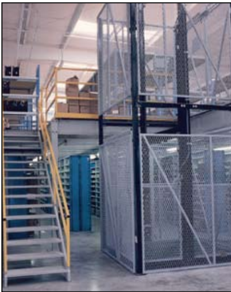
Structural mezzanine combined with vertical lift provides easy movement of palletized loads between levels
