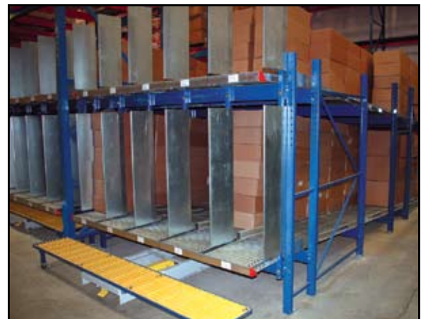
Above: Rear in-feed lanes help keep the cartons aligned for smooth, first-in-first-out flow storage. Step rolls out for easy access, rolls back in to clear the aisle.
