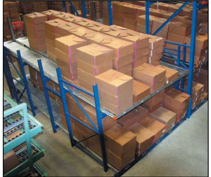
Above: Column flow carton flow racks are perfect for order picking. This allows you to increase the number of carton pick faces in the same space.
