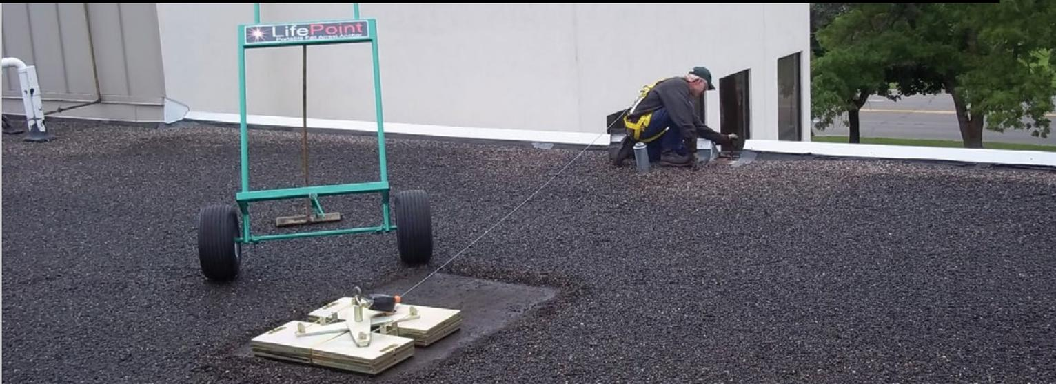
The new LifePoint **Single Tie Off Point (STOP)** is the perfect solution for fall protection when circumstances require non-penetrating versatility. LifePoint provides the answer with an easy to set up and quick-move solution.
