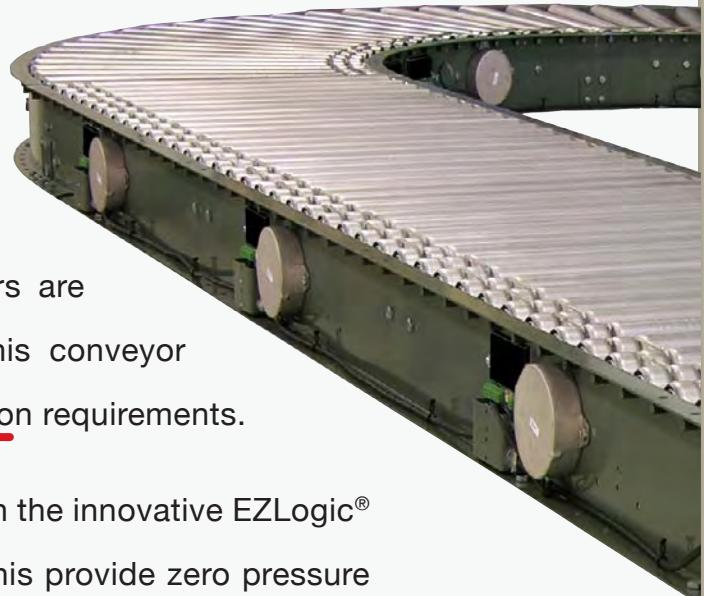
Hytrol has additionally paired the E24™ with the innovative EZLogic® accumulation technology. Not only does this provide zero pressure accumulation but also numerous other functions to the conveyor system. The sleep feature of EZLogic® turns rollers off while not in use, allowing for no energy consumption when product flow is not required. Combining these technologies provides unprecedented flexibility into a highly durable solution.
