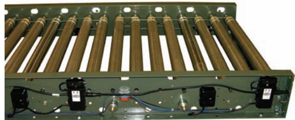
Each zone is powered by a motorized roller. The remaining rollers in that zone are slave driven from the motorized roller with o-rings.
