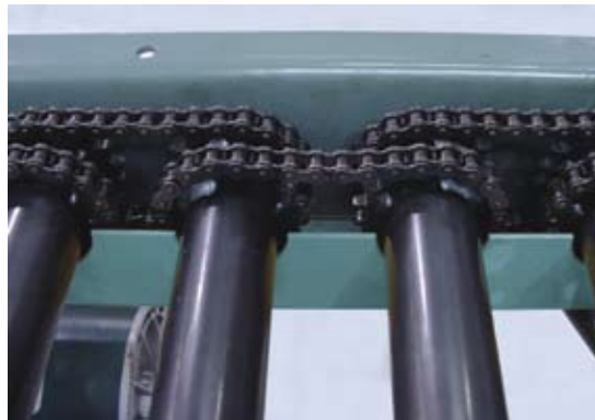
CHAIN GUARD REMOVED TO ILLUSTRATE ROLL TO ROLL DRIVE CHAIN.
