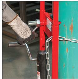
Chain clamping system tightly secures cylinder for lifting and transport
