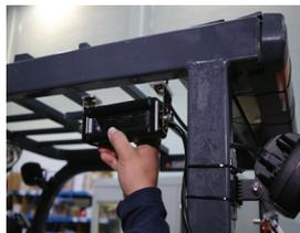
3. Place light near back of over head guard. Ensure the operator can exit and enter the seat without hitting head on light.
