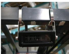
4. Place the two clamps around the over head guard and secure the LED Light feet.
