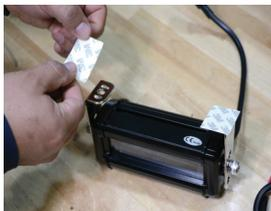
2. Place 2-way tape on feet of bracket. This will reduce vibration and prevent rattling.
