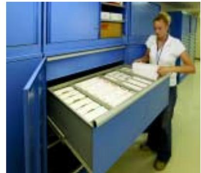
Stacked cabinets with sliding door shelf cabs on top and hinged door cab with drawers (bottom is a 350) and roll-out trays.
