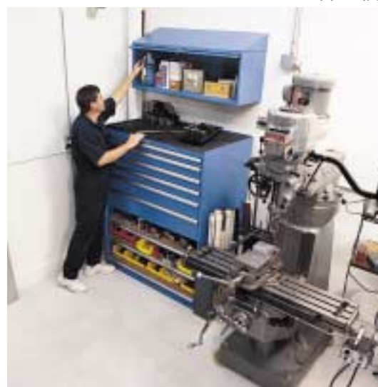
Overhead cabinet with retractable door, drawer and roll-out tray storage in the machine shop.
