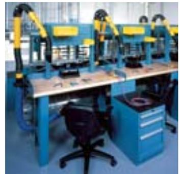
***Lista's custom solution for this manufacturer of silver giftware included workbenches with cut-outs for particle recovery systems and specially-configured companion drawer cabinets.***
