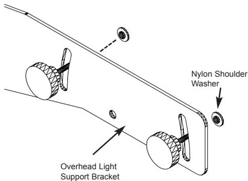
While mounting the pivot bracket to the Flexworks Light bracket, insert a  $\text{Ø}1/4" \times 1/8"$  long nylon shoulder washer into the Flexworks light support bracket. Make sure that the shoulder goes into the crescent moon shape of the light bracket and the flat part of the washer goes between the pivot bracket and the light support bracket, as shown in the figure below.
