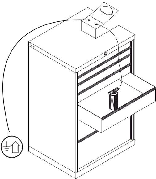
**Resistance to Ground (or Groundable Point)** measures the total resistance between the surface through the ground cord. According to EOS/ESD - S4.1, resistance to ground should be measured using the apparatus listed above with one electrode placed on the surface and the other terminal connected to a groundable point. The resistance should measure between  $10^6$  and  $10^9$  ohms.
