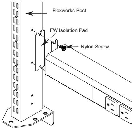
Follow the instructions included with your shipment for installation of the Flexworks Horizontal Power Rail, shown in the Assembly and Use Instructions for Flexworks Accessory System. Include the following steps in your installation to ensure proper isolation.
