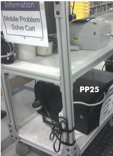
PP25 Stand Alone Power Package shown on bottom of cart
