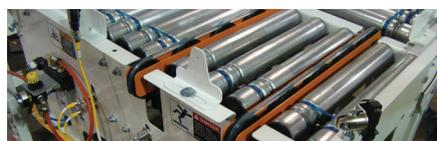
Transfers: Urethane and timing belt, pneumatic and 24V actuated
