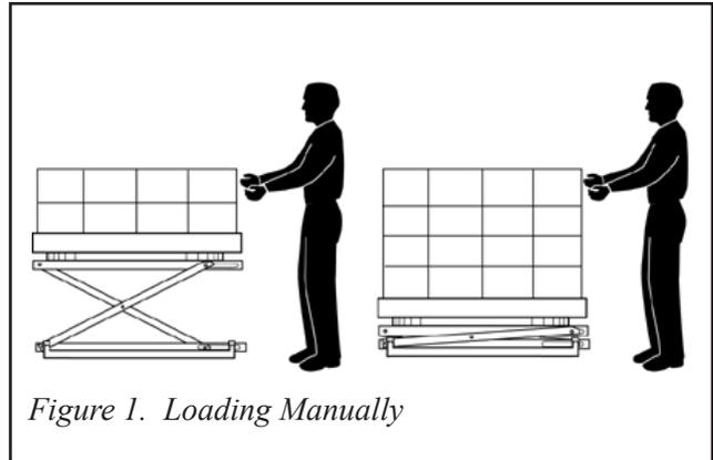
Figure 1. Loading Manually
