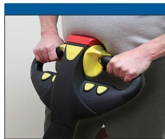
Auto-reversing "belly bump" switch protects against operator accidents while working in tight quarters.
