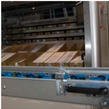
The LogiMat has been provided with a turbo-function, allowing two trays to appear in the pick-window at the same time. Apart from the turbo-function the LogiMat also has a tilting function that lifts the back panel of the tray to provide better overview and ergonomics. The control function of the LogiMat will communicate directly with the picking system of the area, meaning that picking can be done swiftly and without the appearance of any documents.
