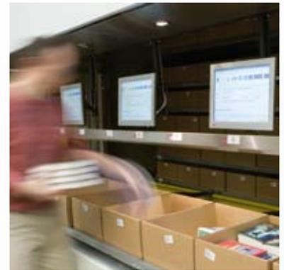
Three flat screens display an identical picture. The screens contain information about ongoing operations, and a light above each individual box indicates the current activity. Once a box has been filled an invoice is printed, the box is dispatched, and a new box will replace the previous box.
