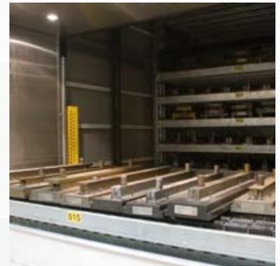
In order to solve the problem Nissens purchased 3 LogiMat vertical lifts where tools are placed on tubular pallets. Once the elevator of the LogiMat has transferred the pallet to the pick-window a lifting device with rollers will appear through the bottom of the pallet.
