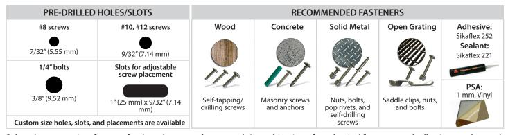
Select the appropriate fastener for the substrate to be covered. A combination of mechanical fasteners and adhesive may be used. Sikaflex 221 sealant may be used to seal edges to deter corrosion. Fasteners and pre-drilled/slotted holes are available upon request.
