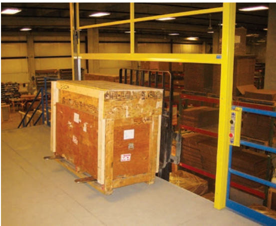
Vertical lift gate
