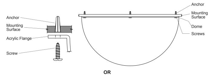
They can also be mounted by pre-drilling holes in the mounting surface and inserting a toggle bolt assembly (not included) through the pre-drilled holes on the mounting surface, then drawing the dome up by screwing the toggle bolt in.
