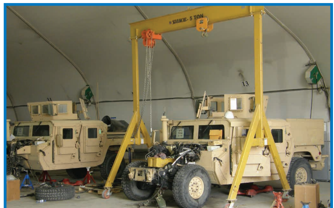
Spanco 5-ton A Series Gantry Crane lifting engines from military vehicles for maintenance.
