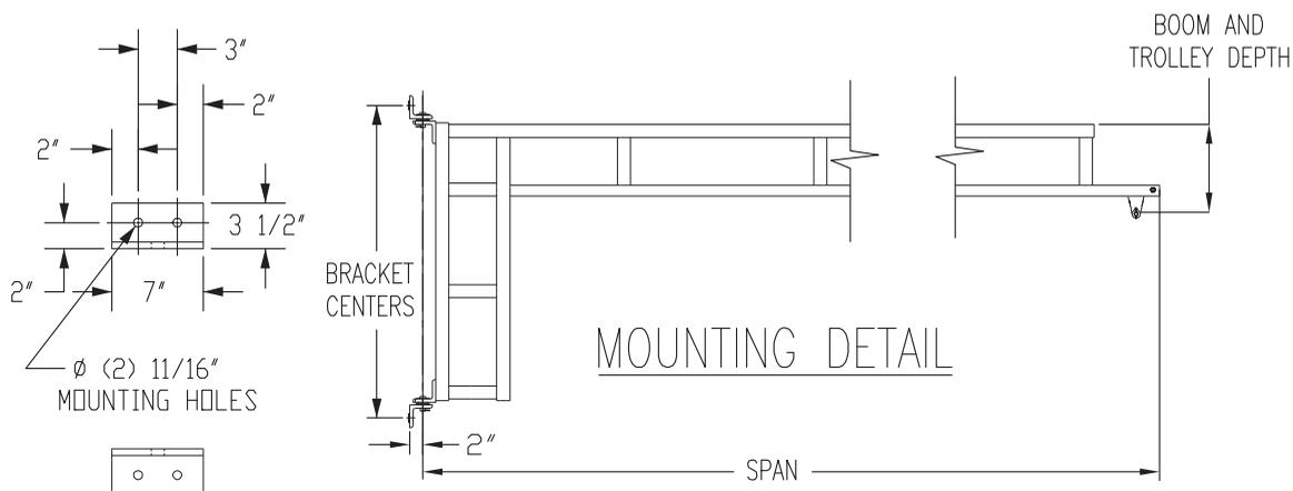
1. Refer to **Tables (1) and (2)** and locate the dimensions of the specific Model WC jib crane to be installed.
