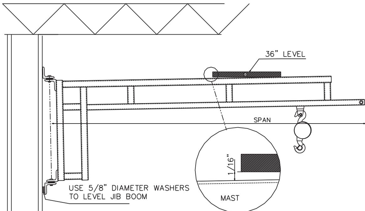
8. Recheck to make sure both upper and lower bearing assemblies will pass the first inspection (see correct figures in this manual). Test jib by rotating back and forth to ensure there is no unusual rubbing or binding or anything else unusual that could compromise the crane, bushings, or pin life. Be sure the crane rotates freely and unimpeded.
