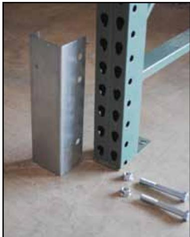
**6.** Select height for the lower mounts that intersects with two of the three holes in the guides and does not interfere with the location where you wish to install the lowest shelf support. Fasten the lower mounts to the rack frame with 4" hex bolts and nuts.
