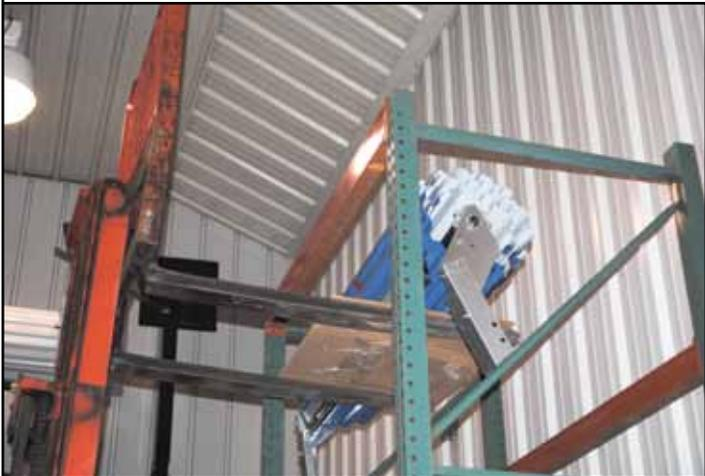
**4.** Lift the door assembly into the rack, and position under the top cross arm of the pallet rack.
