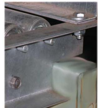
**Knotched** section has end cut to accept beam.
