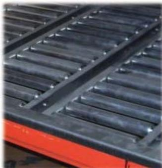
**Hanger** suspends section between front & rear beams.
