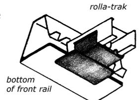
**With guide rail:** The clip is to be installed with its tongue away from the tooth rail, on the one end (only) of the guide rail which sits on top of the teeth. The clip then slides between the teeth and the bottom support ledge of the rail.
