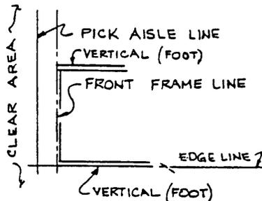
Place one vertical frame flat on the floor, approximately 12" away from the front-line, and with the bottom edge of the frame on the edge-line. Vertical frames have numbered T-slots. Confirm that these numbers are in the "up" position.
