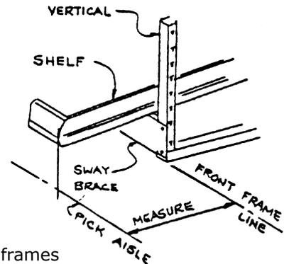
A second set of sway braces should then be attached to the intermediate vertical frame, with the sway braces overlapping and sharing bolts. Plumb and tighten the first set of bolts on the outer vertical frame. Position and bolt on the next vertical frame in the run, repeating the above procedure until all vertical frames and sway braces are in place and aligned on the front-frame line.
