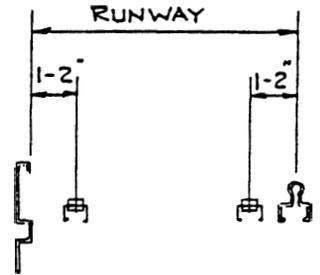
The **Quik-Pik** system is designed to rigidly lock the guide rail at the rear of the shelf, by allowing its shoulder to slip **under** the teeth, while the actual (upper) guide surface passes between teeth. At the front of the shelf the guide rests with the shoulder **on top** of the teeth. Guide rail on some heavy duty shelves, two-piece shelves and/or shelves over 120" long require a plastic clip at the front.
