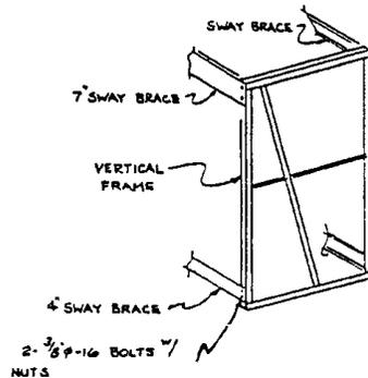
Position a second vertical frame and bolt the sway braces in place, **finger-tight**, using two 3/8" x 3/4" bolts and flanged nuts at each end of each sway brace. These bolts will be tightened later. The **Quik-Pik** shelves are mounted to the vertical
