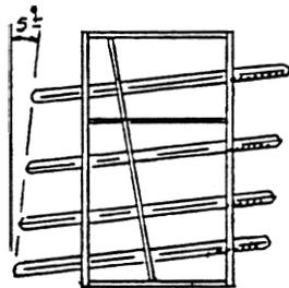
At final installation, all shelves should have a notch over each tab of the rear hanger brackets (two total per side) to prevent forward movement of shelves.
