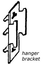
Install one bottom shelf in the section, support with two hanger brackets at the rear and either use hanger brackets or rest directly on the lower sway brace at the front. The shelf should be positioned with the brackets engaging the side rail notches closest to the pick-aisle line.
