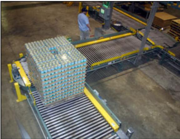
Many operations utilize pallet or slip-sheet to convey bulked material, whether in manufacturing, work in process, to feed a palletizer, or in shipping areas.
