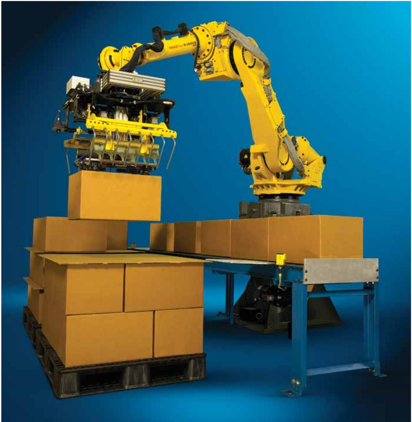
stack with limited shift during shipping. Additional benefits include increased throughput and reduced labor costs compared to manual palletizing. Damage reduction during shipment due to the quality of the palletized load also brings a cost savings while the small foot print such equipment requires opens up floor space for other operations.
