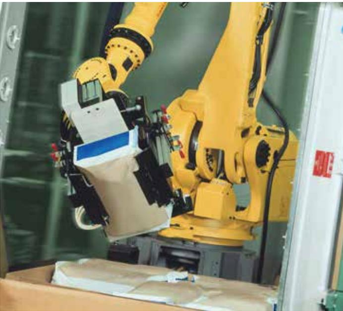
these end-effectors attach to the product and then lift it up. Objects being gripped must have a planar surface in order to assure accurate placement. A vacuum system is required as part of the robotic automation. These grippers require less grasp analysis than many other grippers. Very good for small, lightweight objects.
