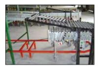
Herringbone Transition centers product onto your flexible conveyor, while floor mounted guide track guides your conveyor under the decline to insure proper storage.
