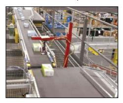
a gap so cases can enter the system individually. The system confirms information such as weight, dimension, data from a barcode and/or RFID tags, or data from vision systems. Based on the data, the case is accepted or rejected, and a number of exception process steps can occur based on your needs.
