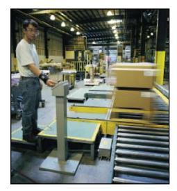
security, safety, and accuracy needs. Example: Our typical high-speed, modular dimensioning system measures products (length, width, height, and volume) on the fly and adapts easily to existing conveyors. If required, it can be combined with barcode scanners and an in-motion scale to capture carton size and weight.
