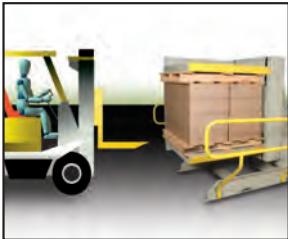
2. Place loaded pallet into rotator/inverter.
