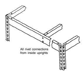
All shelf support (SS) members are 5/16" shorter than nominal length. SS members 42" thru 84" wide have 1 pair of STS rivets at the center line; 96" members have 2 pair of STS rivets.
