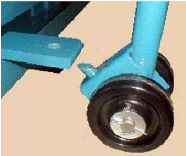
Insert the dolly handle into the tongue on the baseframe
