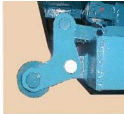
With the platform down, the lift is raised 1" off the floor.
