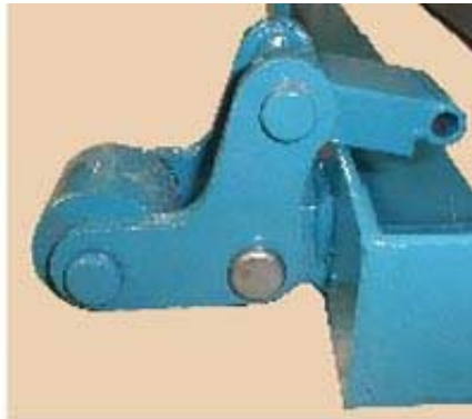
Caster bars in position to raise lift. (BOTH CASTERS MUST BE USED!)
