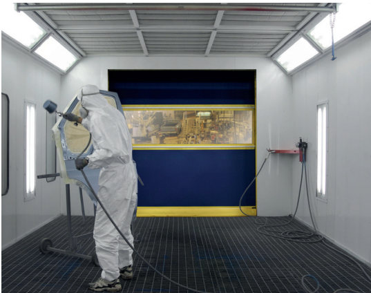
A tight seal means the RR300 can be used to separate clean and dirty environments.
