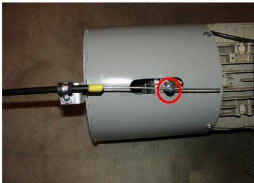
Place exposed end of brake release cable through the thru-hole on brake release arm.
