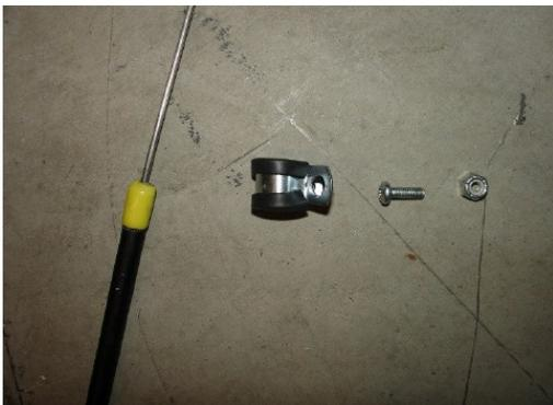
Locate the brake release cable, hose clamp, one 8-32x1/2" bolt and 8-32 Nyloc nut.
