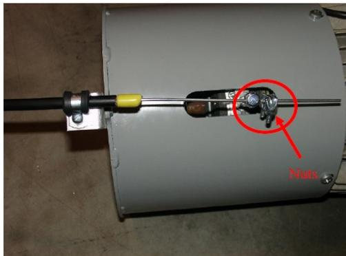
Verify the brake release arm is in the 'Disengaged' or upper position.
