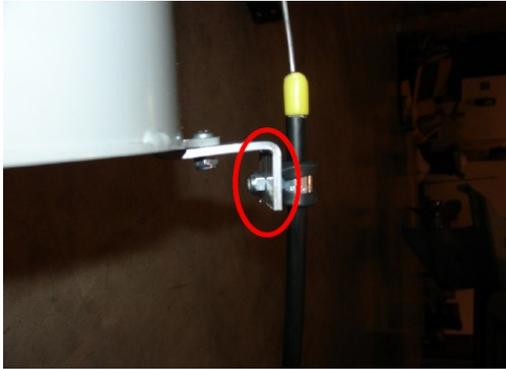
Fasten the 8-32 nut to bolt to secure hose clamp to 'Z' bracket.
