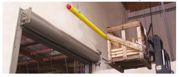
\*To avoid possible false alarms, the Watchman should not be installed, suspended or hung directly from a conveyor structure / frame work.
