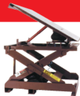
Air Force Lift & Tilt Travel up to 24" Tilts up to 30° Capacities up to 3,000 lbs.
