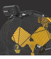
With an effective range of up to 40 ft (12.2 m) within a 90-degree radius, the AirEye Occupancy Sensor automatically turns the fan on to a set speed when it detects infrared motion. Its adjustable lock knob allows users to aim the sensor where airflow is needed most, and two status LEDs display AirEye's power and motion-detection activity. The fan will shut off five minutes after occupants leave the area.
