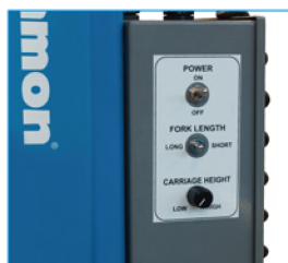
Operator console mounted to back of mast
